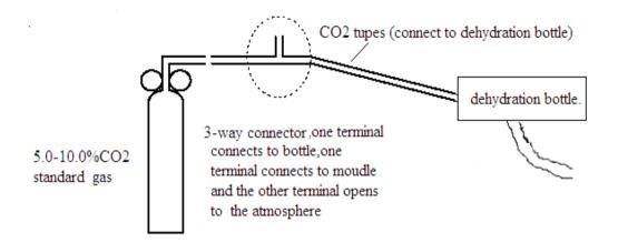
A. Connect the air outlet tubes of standard gas bottle to one terminal of the 3-way connector, and the middle terminal of the 3-way connector opens to the atmosphere; connect the gas sampling tube provided by our Company to the remaining terminal of the 3-way connector (see the circle part of the above figure), connect the other terminal of the sampling tube to the dehydration bottle and the dehydration bottle is inserted into the bracket of the dehydration bottle.
