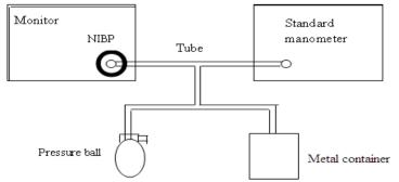
2. Reading of manometer should be 0 before deflate, if not, cut the connection until it return to zero.
