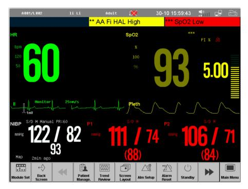
On big numerics screen, you can select any parameters on screen, conduct some parameter settings and observe the parameter as required.
