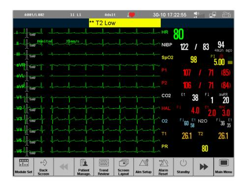
The 12-lead ECG waveforms are displayed in the waveform display area, they are I, II, III, aVR, aVL, aVF, V1, V2, V3, V4, V5 and V6.
