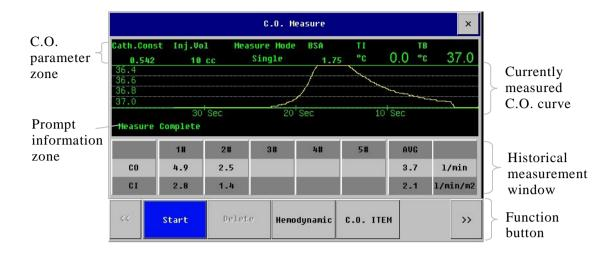
Below the C.O. measurement window, the following function buttons are included:
