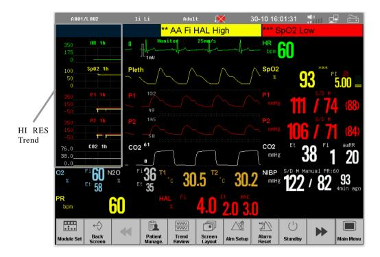
The HI RES Trend graph relevant to the parameters is displayed on the left corner of the waveform, it shows the graphic trend for some time of each parameter. Label and duration of trend display above the each trend, while scale display on the left.
