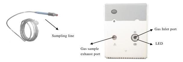
2. Connect the gas sample exhaust port to a scavenging system or return the gas to the patient circuit.
