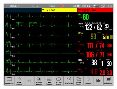
The ECG waveforms of 7-lead are displayed in the waveform display area, they are I, II, III, aVR, aVL, aVF, and V- respectively.
