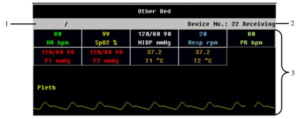
After your monitor is connected to the central monitoring system, you can realize other bed monitoring by selecting the monitors for other beds in the same network. The other-bed-monitoring screen can display all the parameter data of other bed and a certain physiological parameter waveform. You can select at most 10 other-bed monitors to constitute "another-beds-monitoring group".
