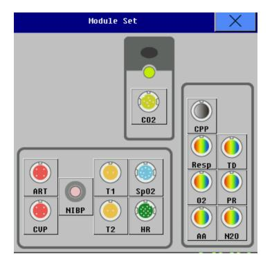
Parameter measurement modules which are configured by user are displayed in above window, and label displays near the corresponding connector of module.
