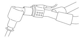
5. Unless the AG sensor is protected with an HME always position the AG sensor with the indicating LED pointing upwards
