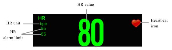
If the monitor doesn't obtain an effective HR value by ECG measuring, the PR value will be displayed instead here.
